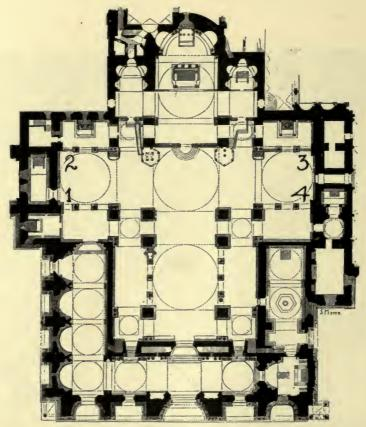
FIG. 5. GROUND PLAN OF S. MARK'S AT VENICE. Showing the conditions of thrust in the nave piers and at the angles 1, 2, 3, 4.
