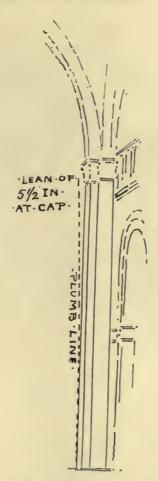
FIG. 14. RIGHT PIER, CHOIR OF S. AMBROGIO. Showing lean of the pier. Compare Fig. 13.
